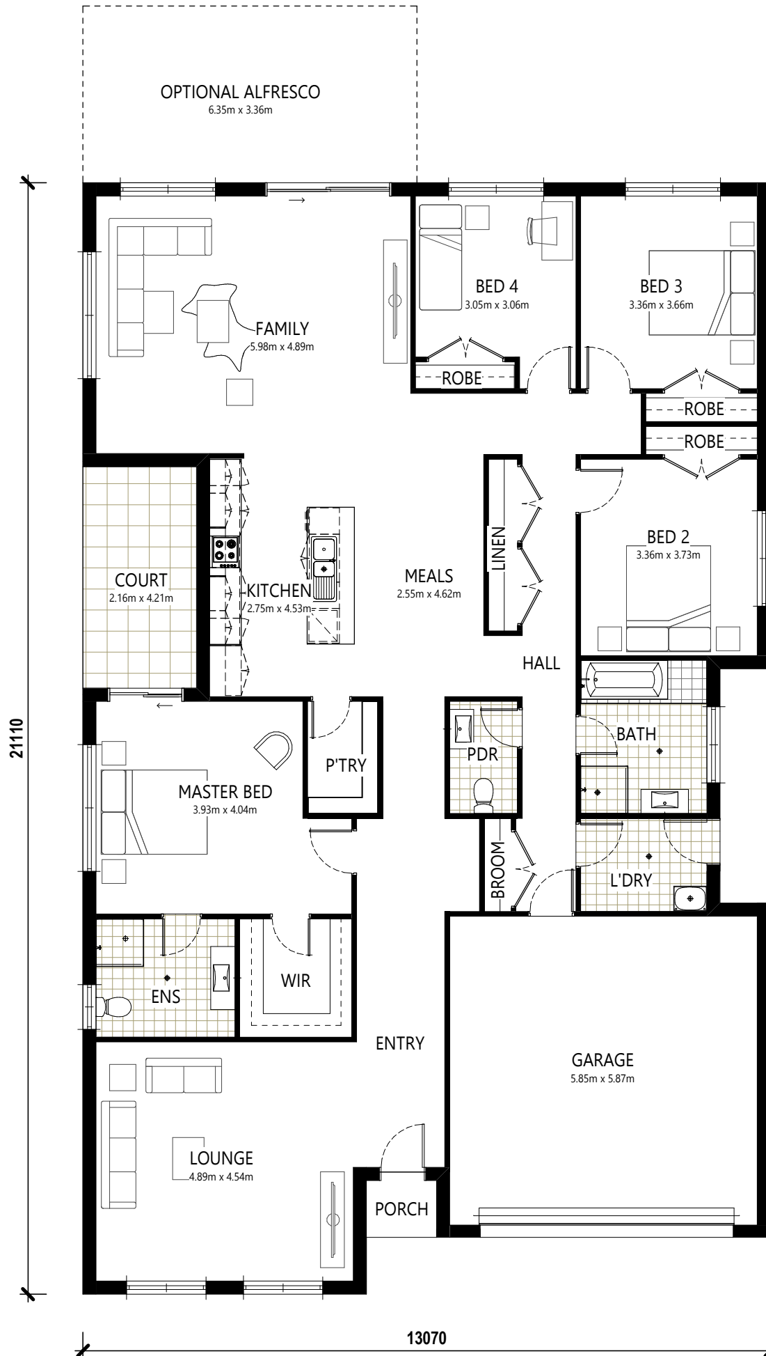
1 FLOOR PLAN SCALE: 1 : 100
